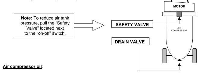
It is very important to maintain the proper oil level at all times. Turn the power to the air compressor off, and then remove the dipstick to check the oil level. If the oil level is "low", add small amounts of oil, secure the dipstick and run the compressor for approximately 1 minute. Repeat the above process until an optimum oil level has been achieved.
