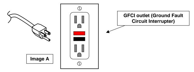
A three-prong cord and matching GFCI outlet (Ground Fault Circuit Interrupter) with a properly installed ground connection must be used with this product (Image A). In addition, the green wire from the control box (Image B) must remain grounded to the frame at all times [External Green Grounding Wire not applicable on all units].
