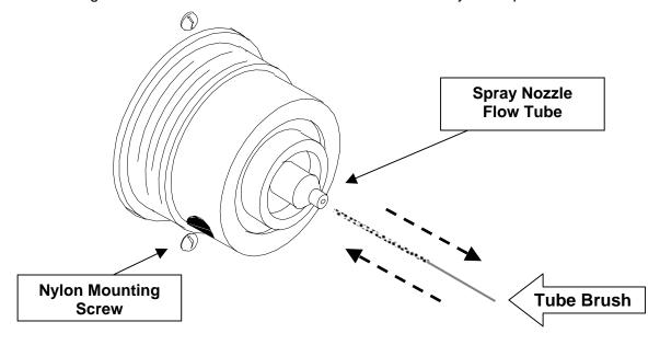
**Step 2.** When replacing the Spray Nozzle Cone, turn the cone clockwise until it begins to feel snug. Align the Spray Nozzle Cone setscrew with the Nylon Mounting Screw located on the spray housing directly underneath the nozzle cone. The setscrew head should be flush against the side of the nozzle cone if properly aligned. Do not over-tighten.
